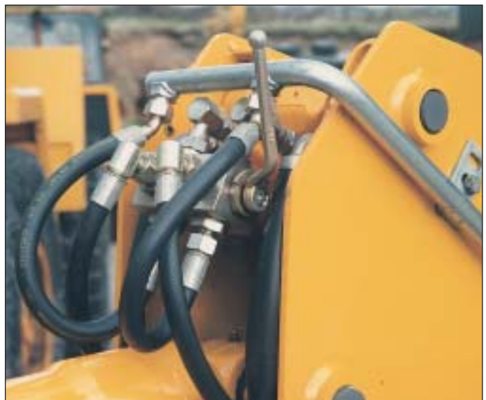
Holmbury HCV6 changeover valve mounted on an excavator arm
